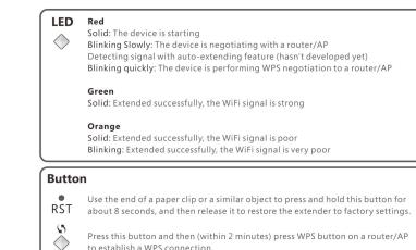
Press this button and then (within 2 minutes) press WPS button on a router/AP to establish a WPS connection.
