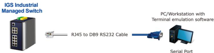
**Figure 4-1:** Industrial L2+ Managed Switch Console Connectivity
