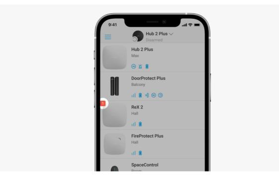
When the range extender detects a malfunction (for example, there is no external power supply), the Ajax app displays a badge with counter in the upper left corner of the device icon.
