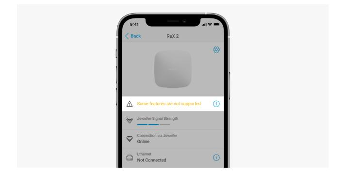
ReX 2 can notify about malfunctions, if any. **Malfunctions** field is available in **Device States**. Clicking on (i) opens the list of all malfunctions. The field is displayed if a malfunction is detected.
