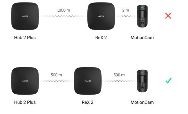
Check the Jeweller and Wings signal strength at the installation site. If the signal strength is low (a single bar), we cannot guarantee the stable operation of the security system. At the very least, relocate the device as repositioning even by 20 cm can significantly improve the signal reception.
