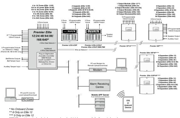
When mixing wired and wireless expanders check total zone capacity for the control panel.
