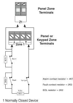
with Fault and Mask (Mask = Fault + Alarm)
