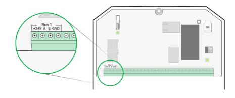
+24V — power supply input A, B — signal terminals GND — ground
