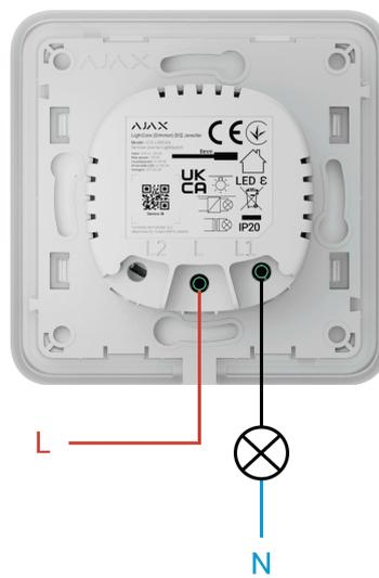
1. Connect the power phase wire to **LightCore (Dimmer)** (terminal L).
