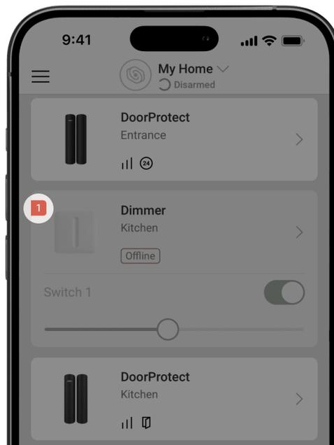
When the switch malfunction is detected (for example, there is no connection with the hub), the Ajax app displays a malfunction counter on the device icon.
