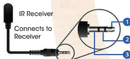
1. IR Signal, 2. Power, 3. Earth
