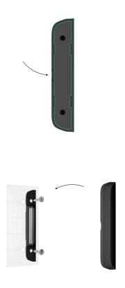
**9.** Tighten the holding screw on the bottom of the detector's and magnet's enclosure. The screw is needed for more reliable fastening and protection of the detector and the magnet from quick dismantling.
