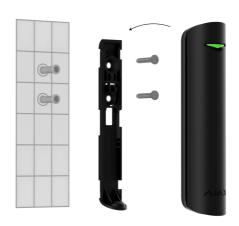
**2. To mount a big magnet**: remove it from the SmartBracket mounting panel.
