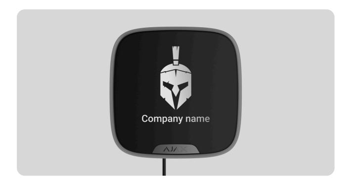
**StreetSiren DoubleDeck Fibra** is a wired siren of the Ajax system with the ability to install a branded faceplate. Equipped with a LED frame and piezoelectric alarm indicator producing sound volume up to 113 dB. For both indoor and outdoor installation.
