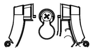
The keyhole fixing is accessed by opening the inner cover as described in the previous section.
