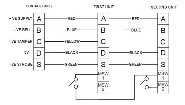
If the first unit is opened it will self-activate and a tamper will be signalled to the control panel. If the second unit is opened both units will self-activate and a tamper will be signalled to the control panel.
