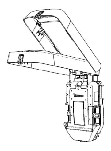
Undo the screw and press the tab to access Wiring & Tamper
