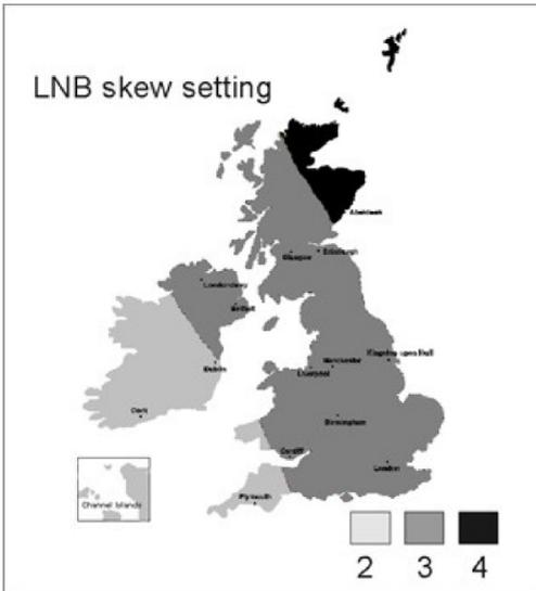
The 3 zones indicated in the illustration above correspond to the numbered skew settings on the LNB casing, only positions 2, 3 and 4 are relevant for the British Isles
