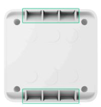
To route the cable from the side, top, or bottom, you can break out any of the six sections at the device's top or bottom or use the side recess highlighted in the picture. Use pliers to break out a section of the device enclosure or drill the hole in the highlighted areas, considering the size of the pipe, corrugated pipe, conduit, or cables.
