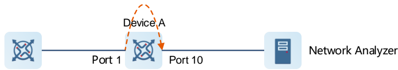
Figure 12-1 Port Mirroring Principles Figure
