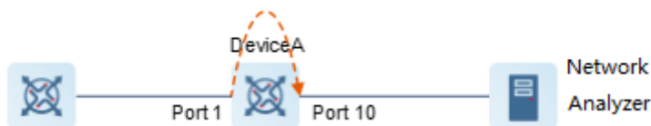
Figure 4-1 Operating Principle of Port Mirroring
