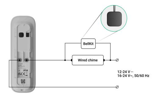
Once DoorBell and BellKit are connected to a wired chime, you need to configure the chime connection in an Ajax app. Before configuring, ensure that DoorBell is **added to the system**.
