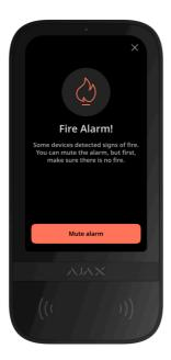
In case of a fire alarm in the system, users can mute it using KeyPad TouchScreen.
