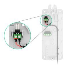
**4.** Once the keypad is <u>installed</u> and added to the hub, check the status of the backup batteries and external power in the Ajax app, as well as the overall operation of the device.
