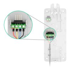
1. If KeyPad TouchScreen is not the last device on the Fibra line, prepare a second cable in advance. Connect the wires to the keypad terminals according to the figure below. The ends of the wires of the first and second cables, which will be inserted into the detector terminals, must be tinned and soldered together, or crimped with a sleeve.
