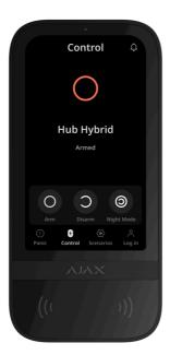
KeyPad TouchScreen can arm and disarm the entire object or specific groups, and activate **Night Mode**. Use the **Control** • tab to change the security mode. Users can control the security using KeyPad TouchScreen through:
