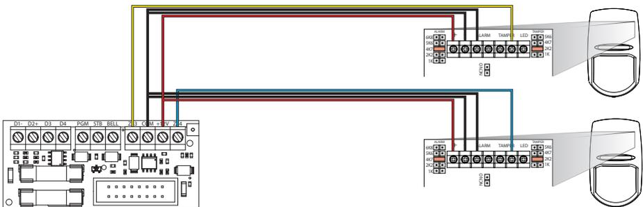
The End of Line (EOL) value for all wired zones is programmed in 'Choose Mode'. At default the resistor values are 4k $\Omega$  for alarm and 2k $\Omega$  for tamper.
