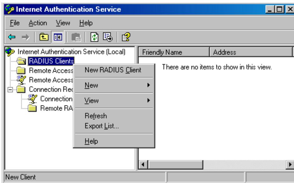
2. Enter a RADIUS client name (which can be the name of the AP) and the IP address of the AP, and click **Next**.
