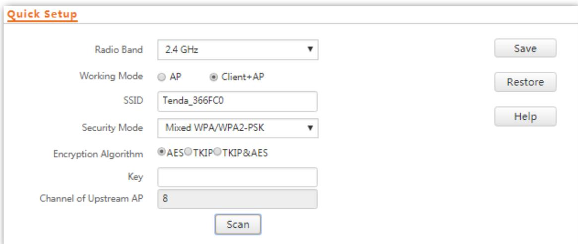
**Step 9** To extend the WiFi network at 5 GHz radio band, select the radio band, and repeat **steps 3-8**.
