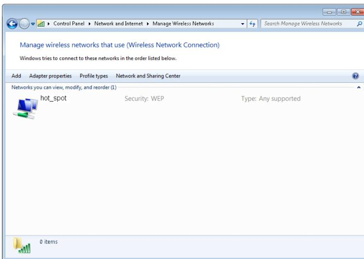
**Step 12** Click the network icon in the lower-right corner of the desktop and choose the wireless network of the AP, such as **hot\_spot** in this example.
