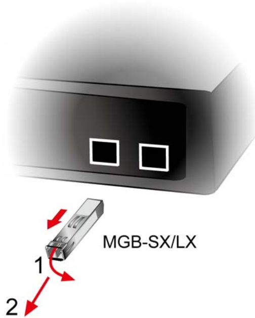
Figure 2-1-8 How to Pull Out the SFP Transceiver
