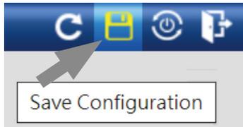
2. Press the **"Apply"** button to save running configuration to start up configuration.
