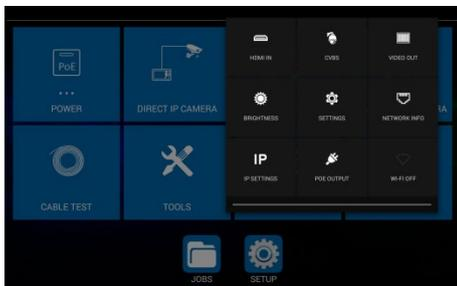
Drag down from the top right hand corner of the screen to reveal the Quick Access Menu. This provides quick access to a selection of commonly used tester functions. (Note that this selection is not user-configurable.)
