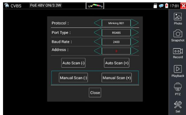
Set protocol, communication port, communication rate, to match the PTZ camera under test, then to press "Scanning" to start the PTZ camera's address searching.
