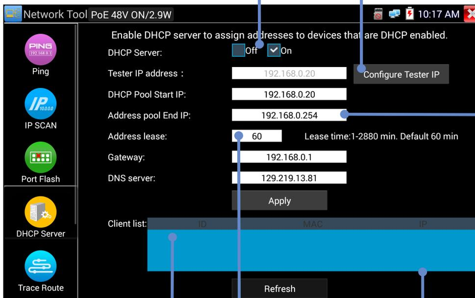
Set up a pool of addresses that the DHCP server can assign
