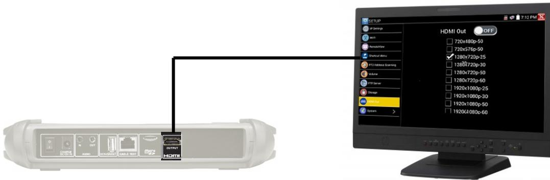
Tap to switch the HDMI output on/off (default is ON)
