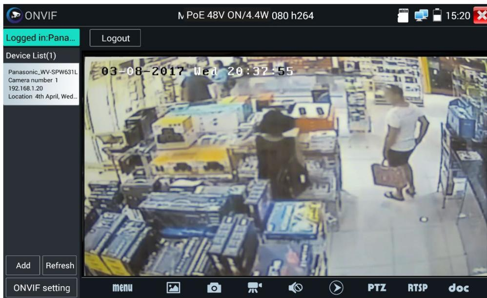
If the camera is disconnected, tap Refresh to re-connect :
