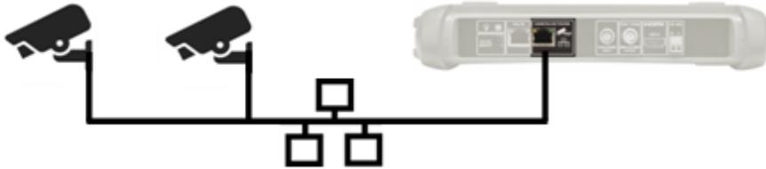
Cameras that are compliant with the standard methods of communication established by the Open Network Video Interface Forum (ONVIF) can be connected and tested without the need to make any manual adjustments to the connection details regardless of camera brand. (Note that some cameras may be only partially ONVIF compliant)
