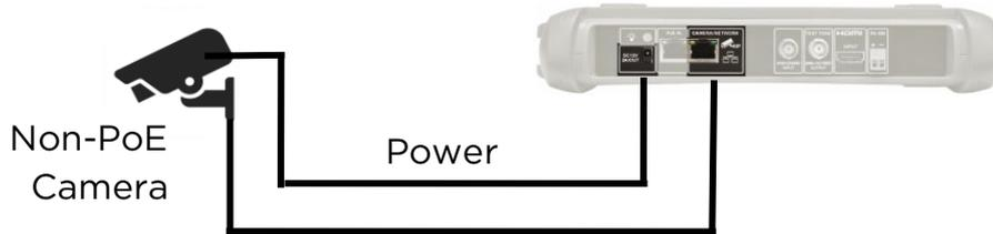
Note that the power is always present on the socket, regardless of the setting of the PoE switch.
