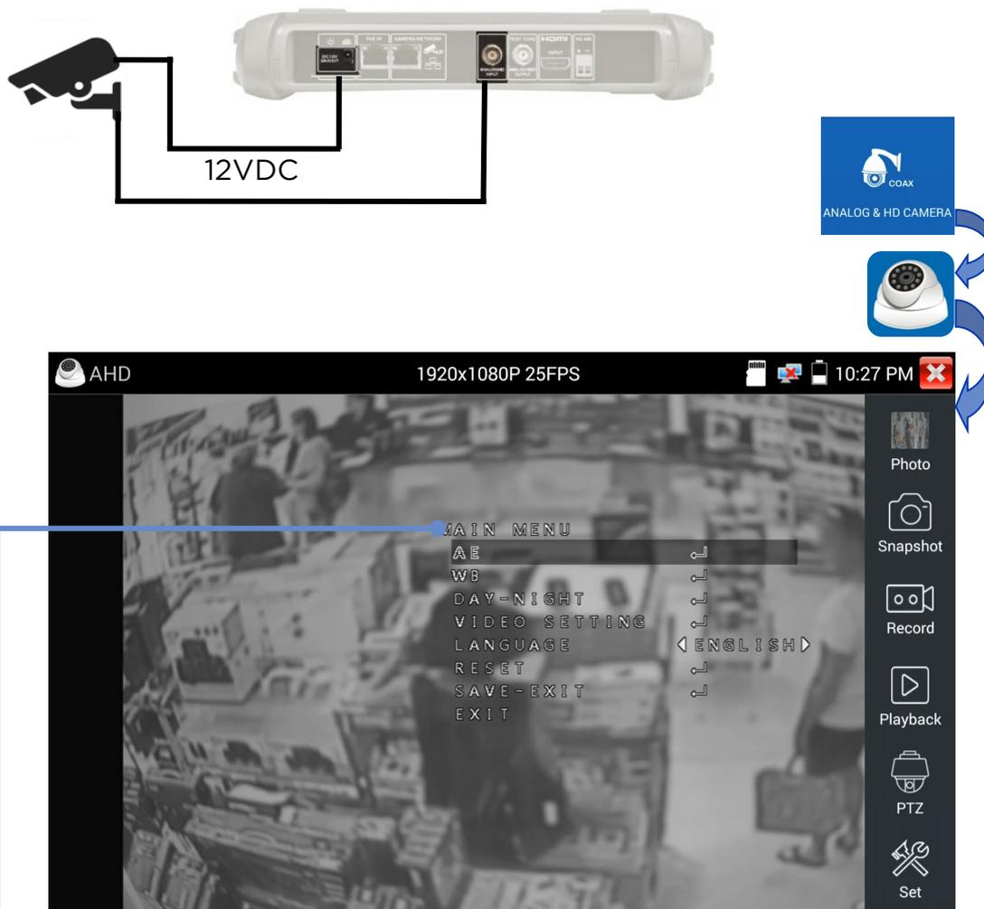
● Navigate and use the camera-based settings menus with the On Screen Display (OSD) menu navigation controls. (Also supported on TVI, CVI and Coax cameras.)
