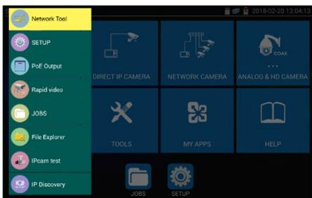
Press the key to reveal the Shortcut Menu. This provides shortcuts to up to 8 tester functions, configurable under SETUP >> Shortcut Menu.
