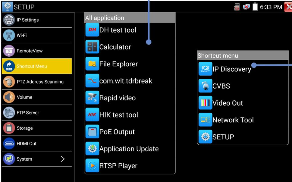
Touch and hold an application to move it back automatically to the main applications list
