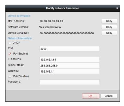
Figure 2-9 Modifying the Network Parameters
