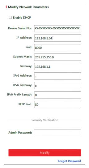
Figure 2-5 Modify the IP Address
