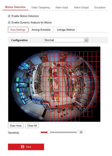
Figure 5-44 Motion Detection Settings
