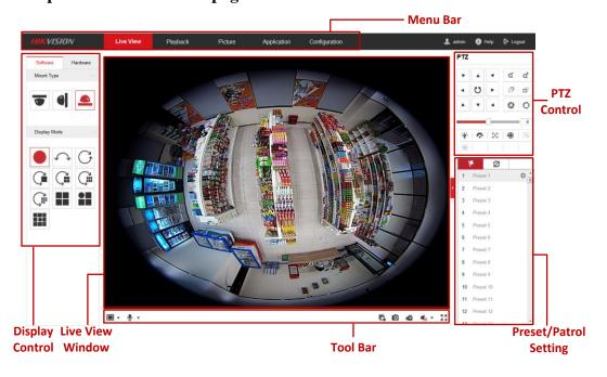
Figure 4-1 Live View Page (Software Decoding)
