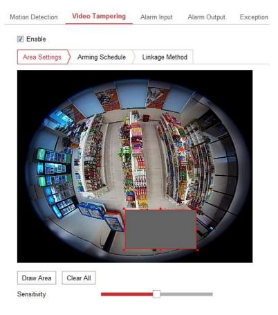
Figure 5-48 Video Tampering Detection Settings
