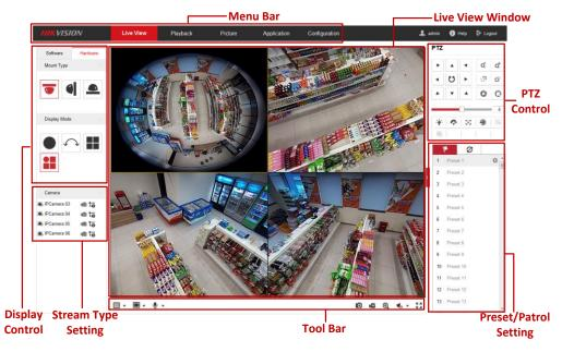
Figure 4-2 Live View Page (Hardware Decoding)
