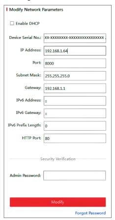
Figure A.1.2 Modify Network Parameters
