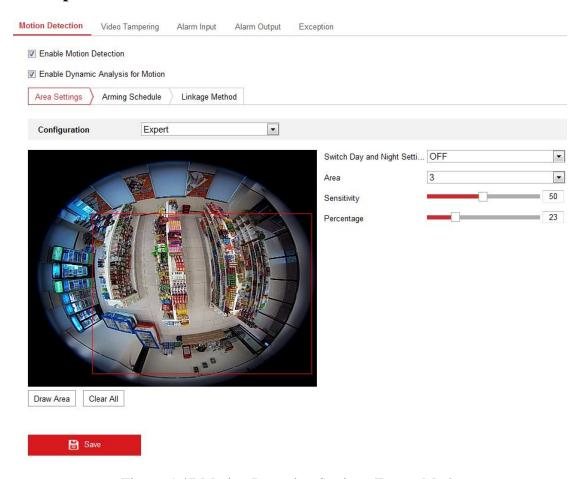
Figure 5-47 Motion Detection Settings-Expert Mode
