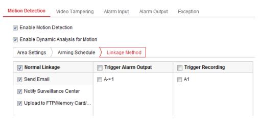
Figure 5-46 Linkage Method Settings
