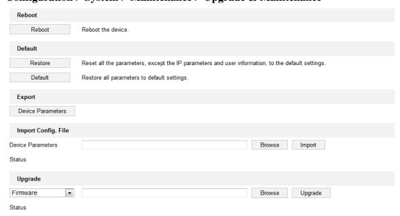
Note: The upgrading process will be 1 to 10 minutes, please don't disconnect power to the device during the process. The device reboots automatically after upgrading.
