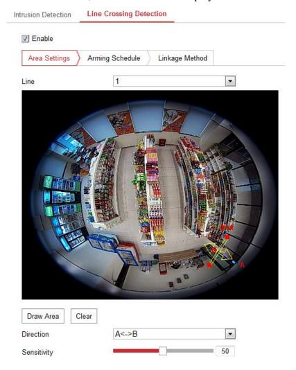
Figure 5-52 Line Crossing Detection Setting
