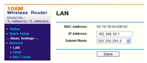
Figure A.2.2 Set the LAN parameters
