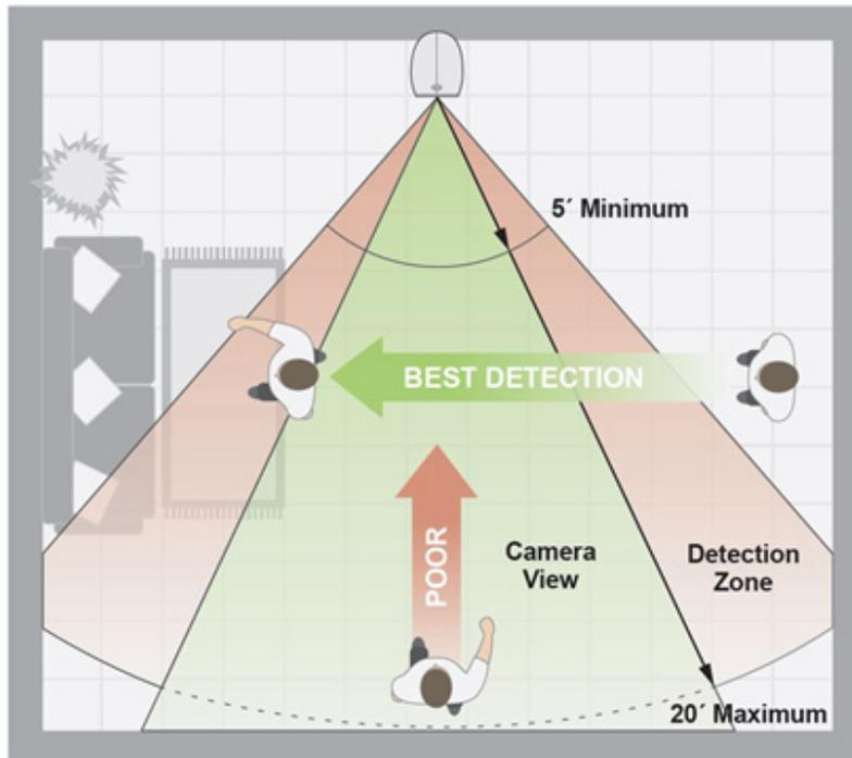
You can use the Motion Detection Test feature to verify if motion can be detected in a camera's current placement. The camera's LED blinks amber when motion is detected. Go to your camera's **Settings** option to turn on the Motion Detection Test feature.
