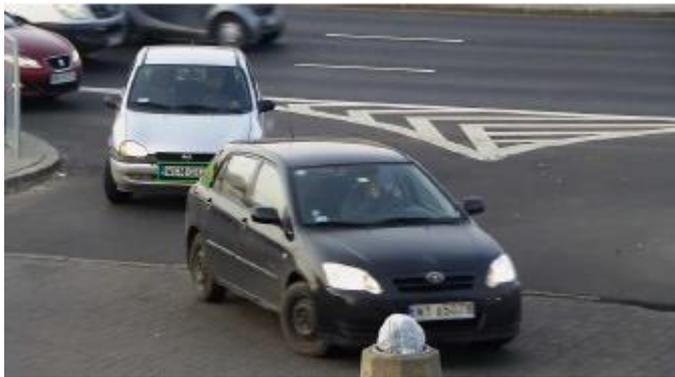
**Solution:** Notice how there is not enough focus for all frame. Car with a green frame will be detected, and other cars will not. Adjust the focus on the lens.
