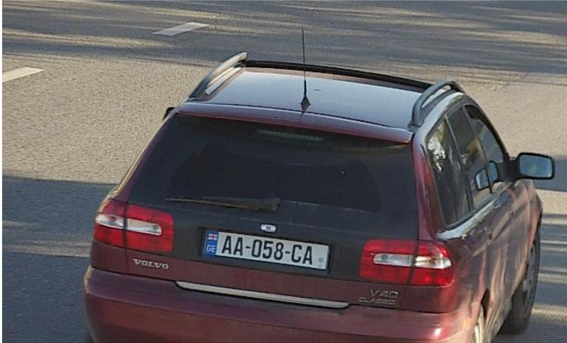
**Solution:** Notice the license plate tilt angle. License plate tilt angle must be within +/-5 degrees.
