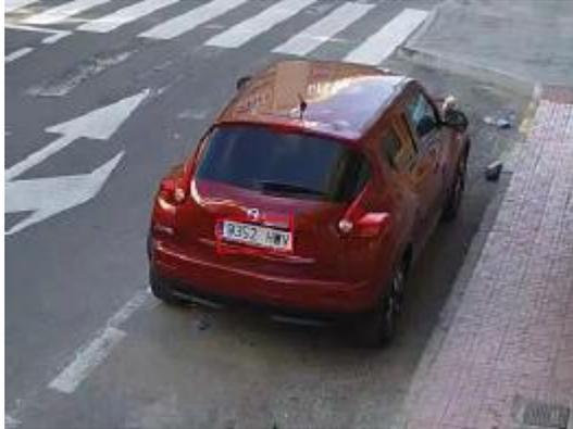
**Solution:** It seems that LP is well lit and readable by eye. However, if we'll measure full frame in photoshop, we will see that LPR width is under 100px which is not enough. License plate width in the frame should be increased and be at least 130 pixels.
